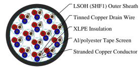
Tinned Copper Drain Wire **XLPE** Insulation Al/polyester Tape Screen
